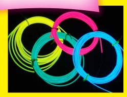
4: When the EL wire is attached to a power source, such as a battery, it glows! A battery pack that powers the EL wires is hidden on each creature in the show.
